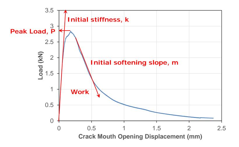
Fracture Energy, G<sub>f</sub> = Work / Fractured Surface Area
